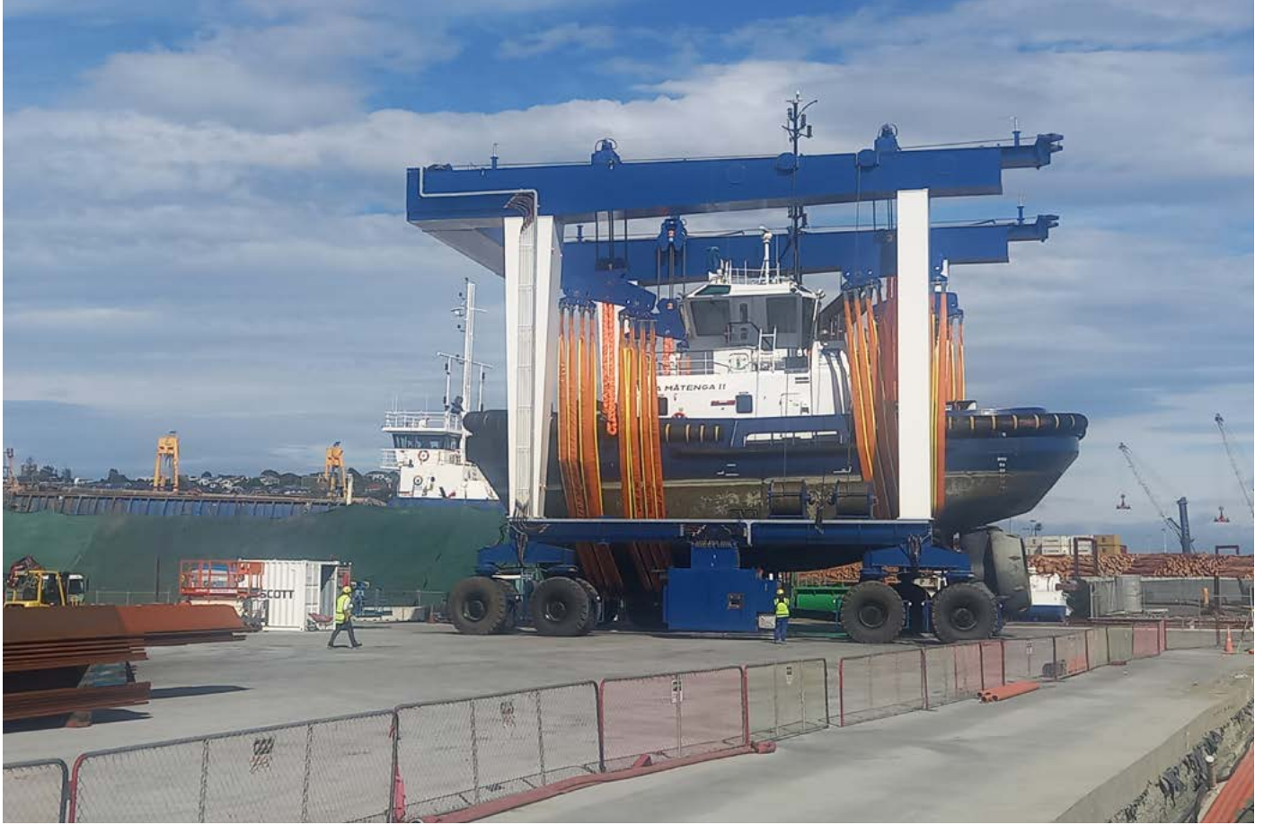
Travel lift in operation at Port Nelson. Photo provided by Kernohan Engineering; Credit: Tim Cuff
